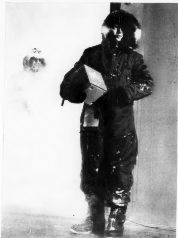
ENVIRONMENTAL TEST CHAMBER simulates atmospheric conditions found at altitudes up to 100,000 feet.
